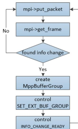
Figure 15 Semi-internal allocation mode decoder work flow
