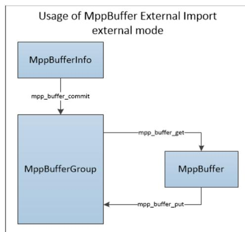
Figure 5 Usage of MppBuffer External Import
