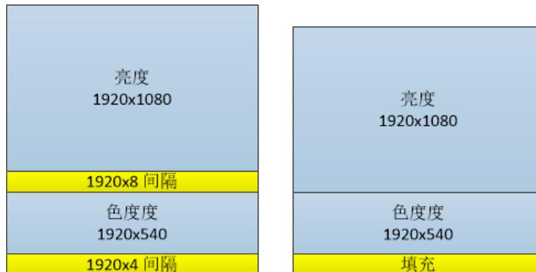
Figure 18 Encoder input frame memory arrangement
