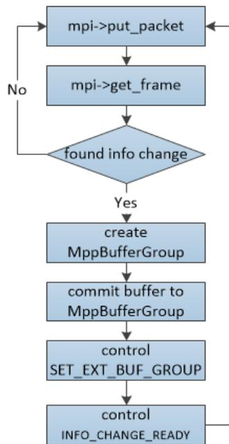
Figure 17 Pure external allocation mode decoder work flow
